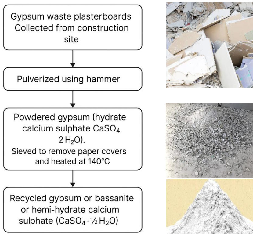
Figure 2. Procedure for the preparation of recycled gypsum
