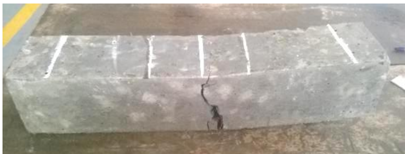
Figure 6. Crack pattern of fiber reinforced self-curing concrete after flexural test
