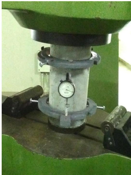
Figure 8. Modulus of elasticity test set up of self-curing concrete
